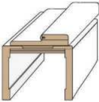
Single Rabbet Telescopic Jamb with Rubber Seal and L-Shaped Casing on Both Sides. Extension is Optional.
