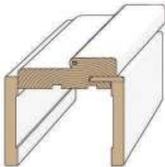
Single Rabbet Half Telescopic Jamb with Rubber Seal, Flat Casing on One Side and L-Shaped Casing on the Other Side. Extension is Optional.
